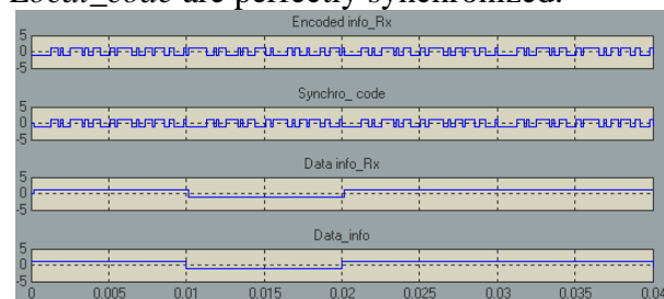
Fig. 4 Waveforms for Encoded info_Rx , Synchro_code and Data info_Rx compared to Data_info for ideal case.
